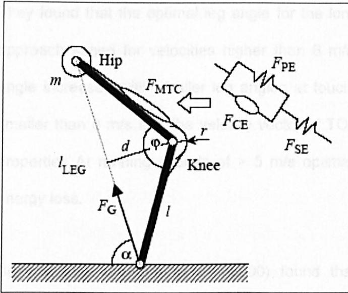
Figure 2.6 Schematic drawing showing the planar spring-mass model
