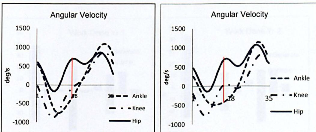
Figure 7.5 Mean angular velocity at ankle, knee and hip from TD to TO in Yr 1 and Yr 2 (the vertical line indicates MKF). All joint angular velocities flexion (-) and extension (+).
