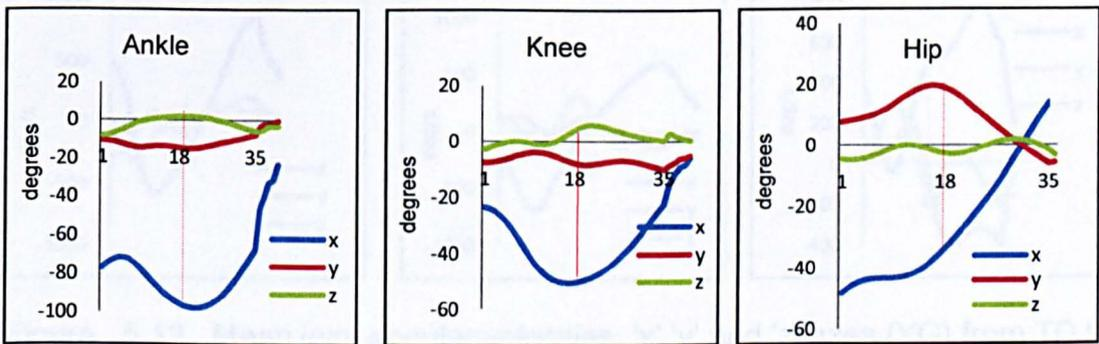
Figure 5.10 Mean joint angles: 'x', 'y' and 'z' axes (YG) from TD to TO (the vertical line indicates MKF). All joints, extension (+), adduction (+) and internal rotation (+).
