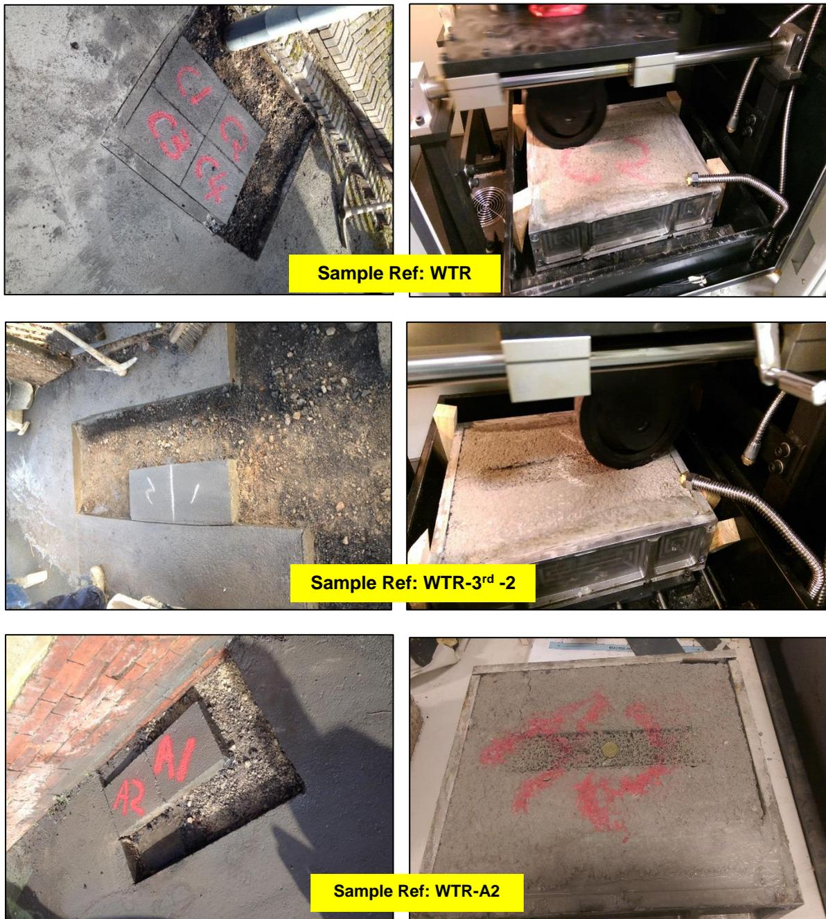
**Figure 7:** Specimen extraction and testing in wheel tracking apparatus
