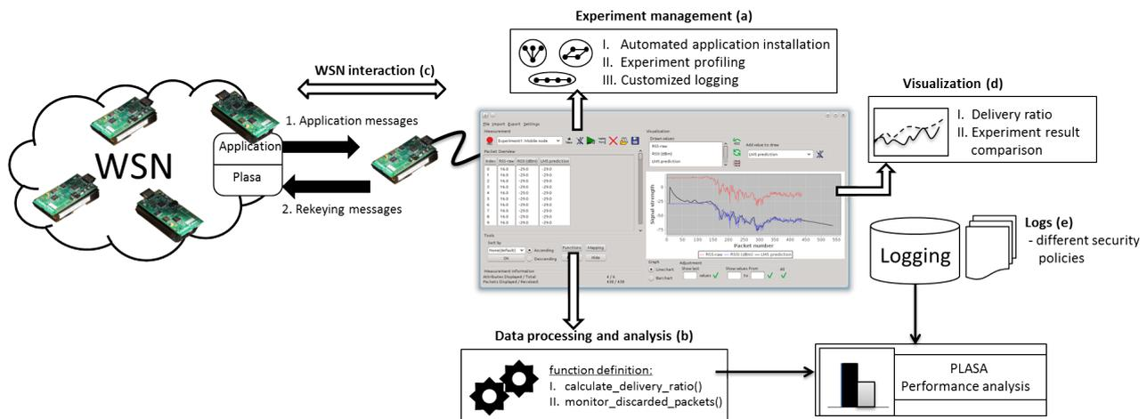
Figure 8. Case 2: Secure communication experiments using IRIS
